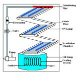
Figure 1. Diagram of experimental photo-degradation reactor
